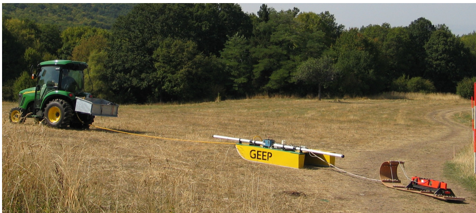
Figure 1. Mobile geophysical platform: EM31 (1 st sledge) and EM38DD (2 nd sledge) are towed by a tractor.
